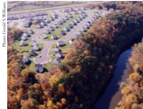
Photo: Gerald S. Williams Residential subdivisions with wide streets are an example of added impervious surfaces that cause cumulative effects throughout the watershed.
